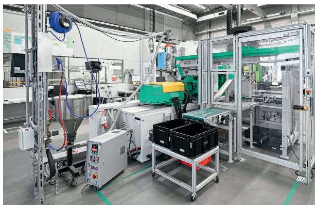
Fig. 2. The turnkey system is energy efficient and can produce nano push button switches flexibly. The Multilift V robot system (right) lays the finished parts aligned on a conveyor belt. © Arburg
