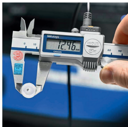
Fig. 1. The nano push button switches save room, are secure, and can be used anywhere. This flagree component is about 12.5 mm in diameter and has a magnet at its center. © Arburg
