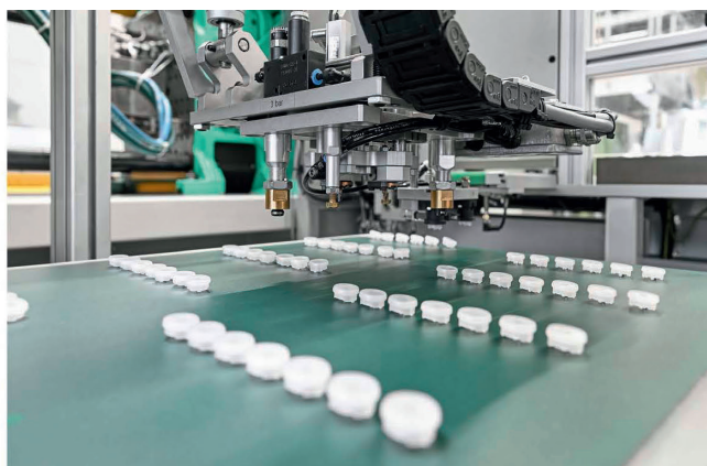
Fig. 2. The turnkey system is energy efficient and can produce nano push button switches flexibly. The Multilift V robot system (right) lays the finished parts aligned on a conveyor belt. © Arburg
